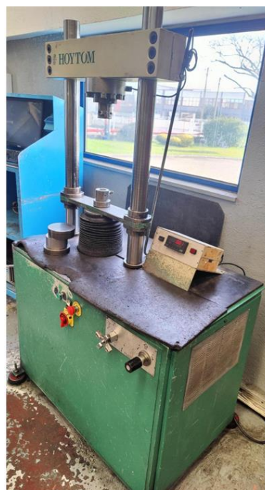
Figure 21 – Rupture test HOYTOM press machine.
