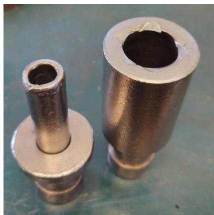
Figure 22 – Punch and tube for the rupture test of the component.
