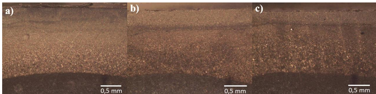
Figure 37 – Electrode’s Wear Study: Weld Nuggets Macrographs with the interface in detail: a) 0 welds; b) 2500 welds; c) 5000 welds.
