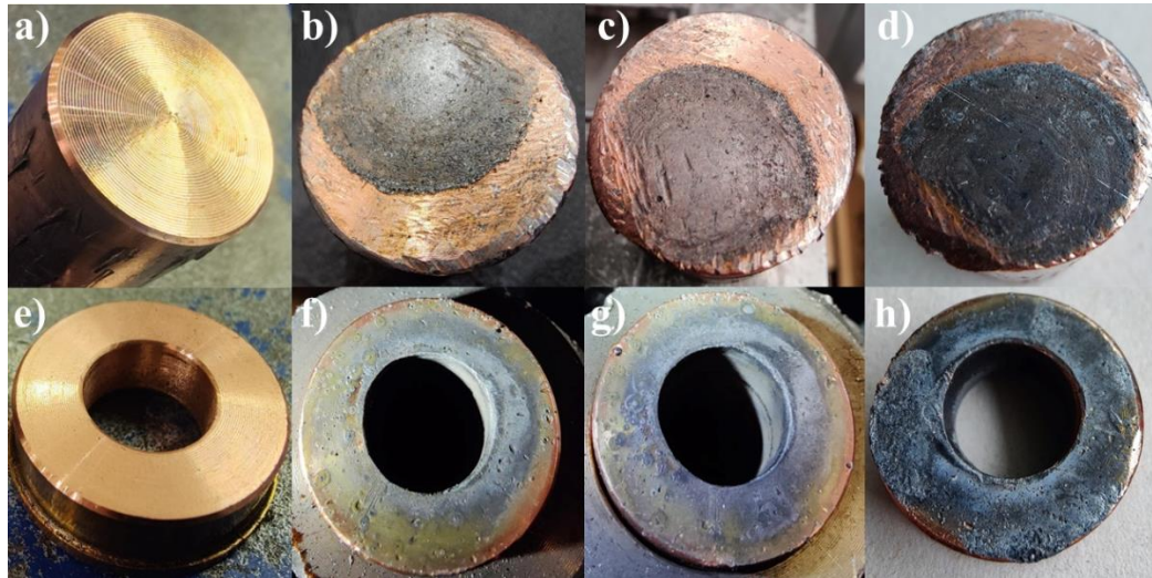
Figure 44 – Electrode's Wear Accompaniment Study: a) and e) 0 welds; b) and f) 2500 cycles; c) and g) 5000 welds; d) and h) 8000 welds.
