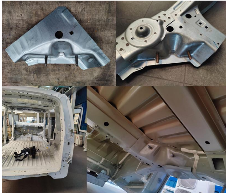
Figure 14 – Zone and cars where the part is assembled on the car structure.
