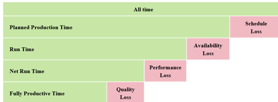
Figure 4 - OEE calculation diagram (in https://www.oeefactors.com/oeefactors/ , accessed in 2023-04-10)
