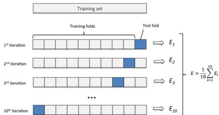
Figure 2.7: An example of a 10-Cross fold validation evaluation method. Adapted from Johar M. Ashfaqe Maat et al Introduction to Support Vector Machines and Kernel Methods
