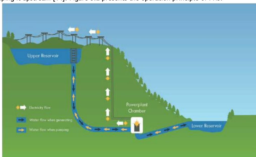
Figure 3.2 - Working principle of PHS [12].
