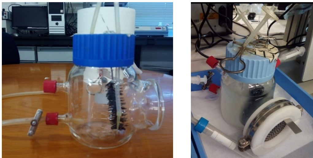
Figure 34: B-MFC used in the experiments; left – Anodic chamber with the anode electrode, carbon brush; right – B-MFC after assembly, with the MEA.
