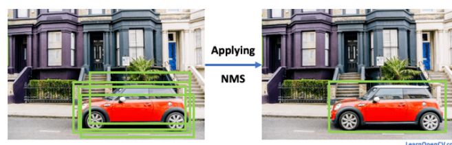
Figure 2.15: Example of Non Max Suppression (adapted from [65]).
