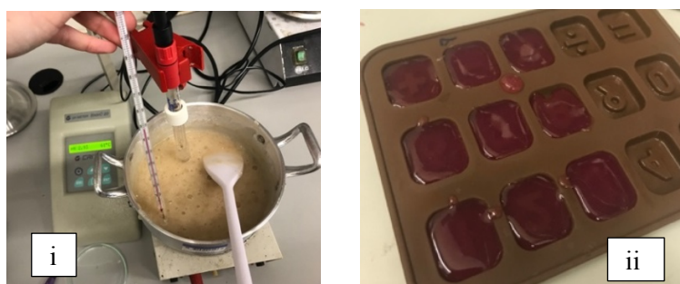
Figure 15 Temperature and pH measurement in a pectin formulation (i) and molding (ii)
