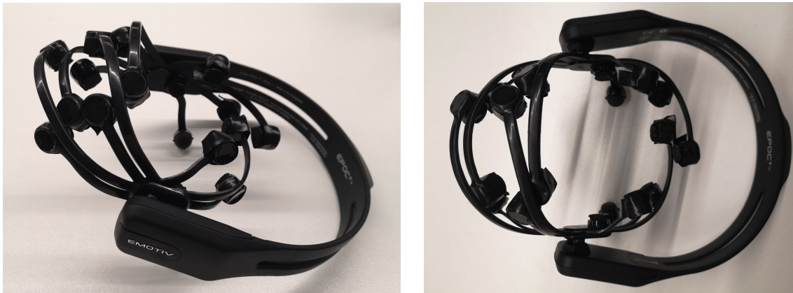
Figure 3.4: Emotiv Epoc+ hardware (from [25]).
