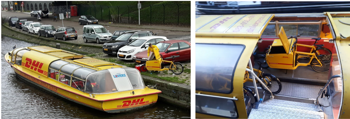
Figure 3.8: DHL's barge meeting up with a delivery bicycle and cargo-cycles stored inside the barge (Parr, 2017a).
