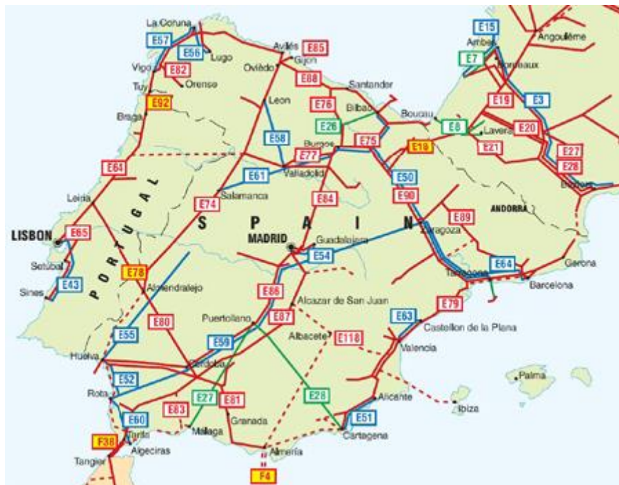
Figure IV-2 - Pipelines network for natural gas (red), oil (green) and products (blue) transport and supply in Portugal and Spain. Source: Theodora database [95].
