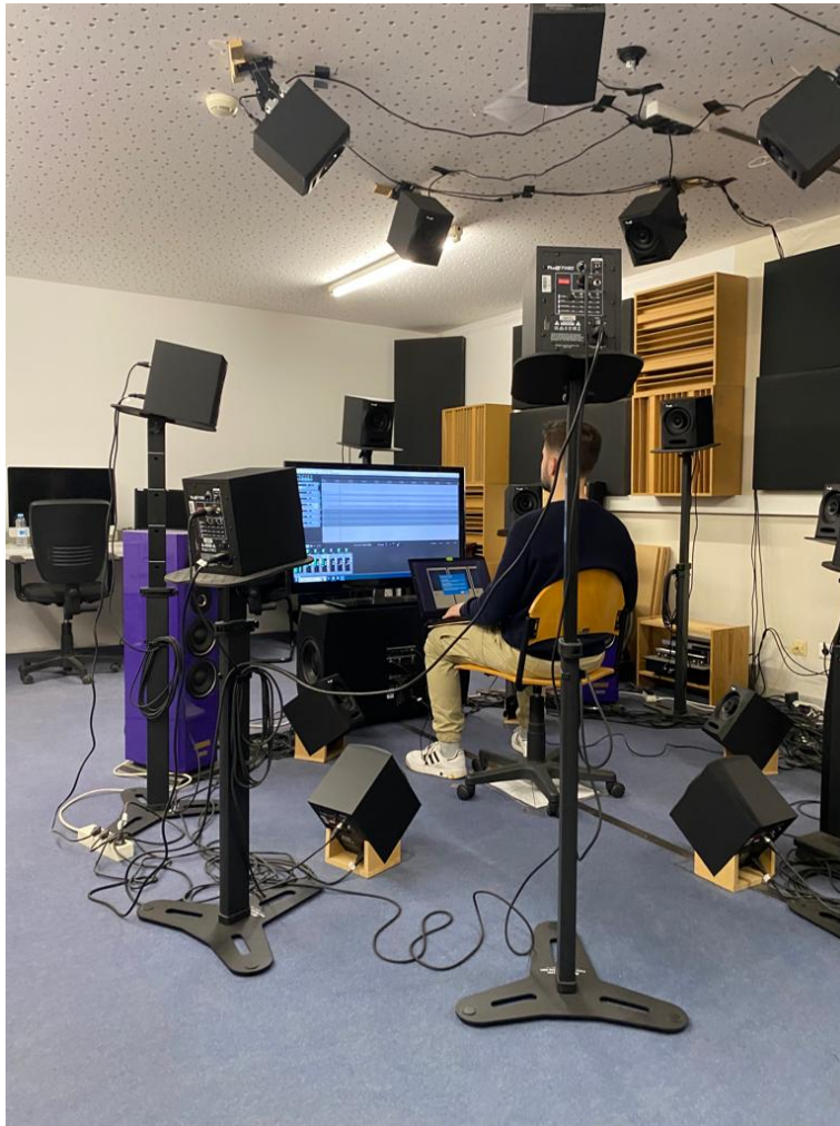
Figure 3.4: Photograph of the multi-speaker array system used in the perceptive analysis.
