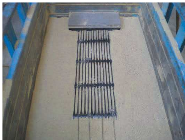
Figure 2. Instrumented geogrid specimen installed over compacted soil.
