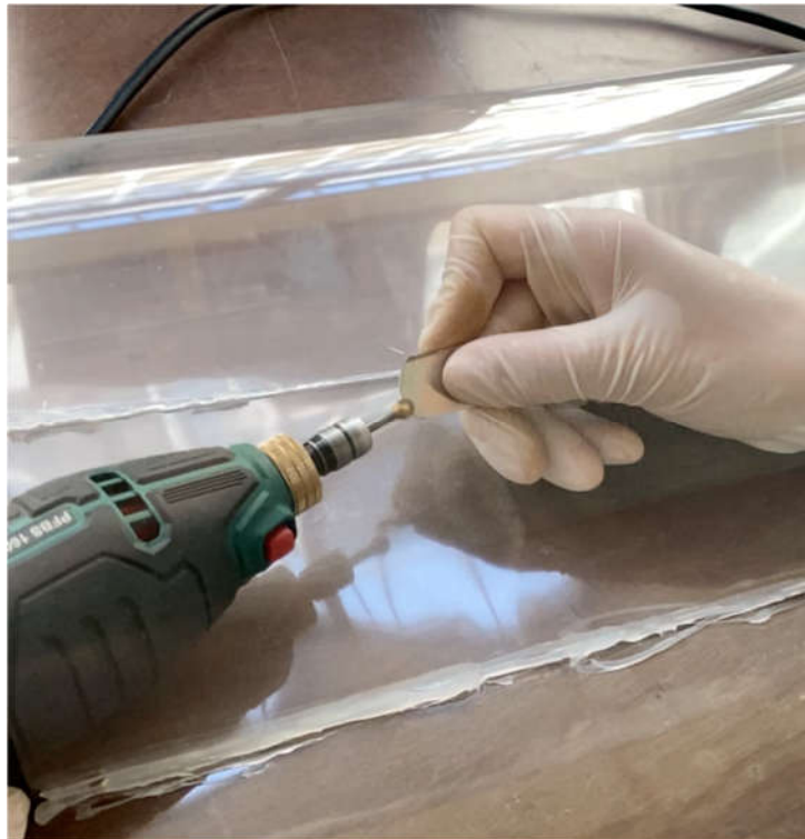
Figure 2.3 – Milling process. The files are shot in every direction, so a transparent cover is used to keep them contained.
