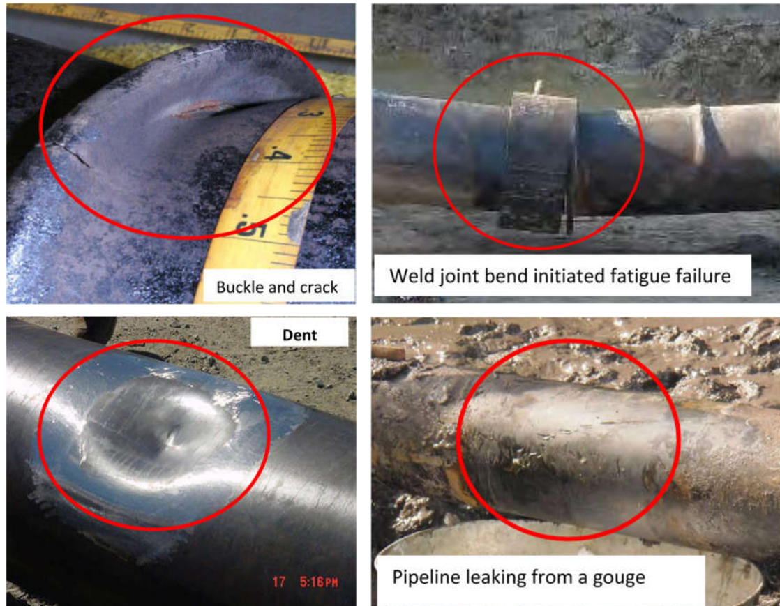
Figure 1.2 – Examples of defects that can be found in pipelines (adapted from [11]).
