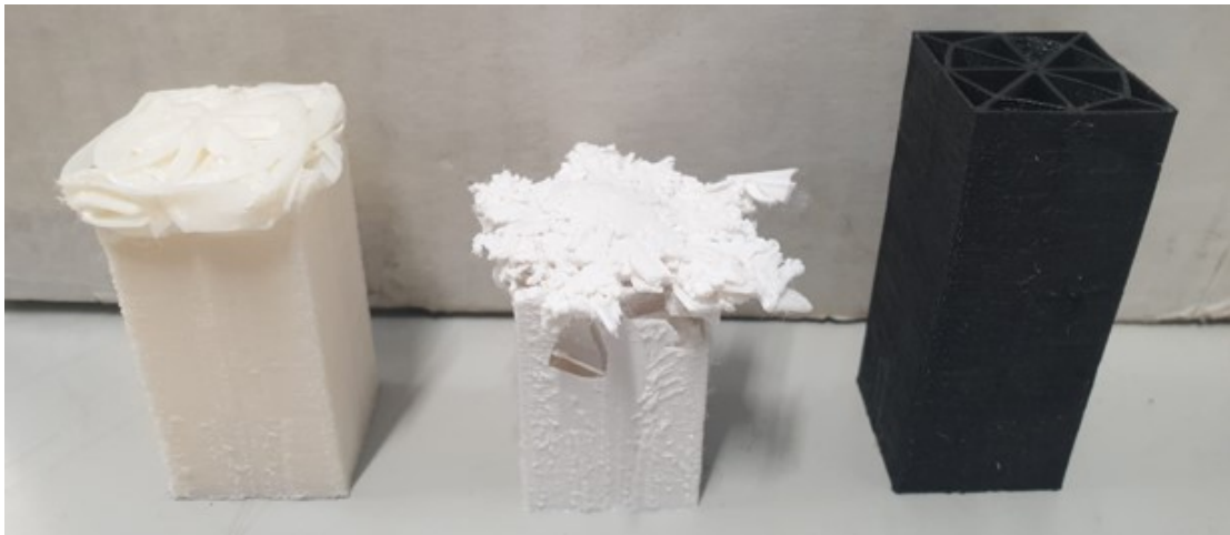
Figure 17: Spider web graded structures after impact: PC (left), PETG (middle), TPU (right).
