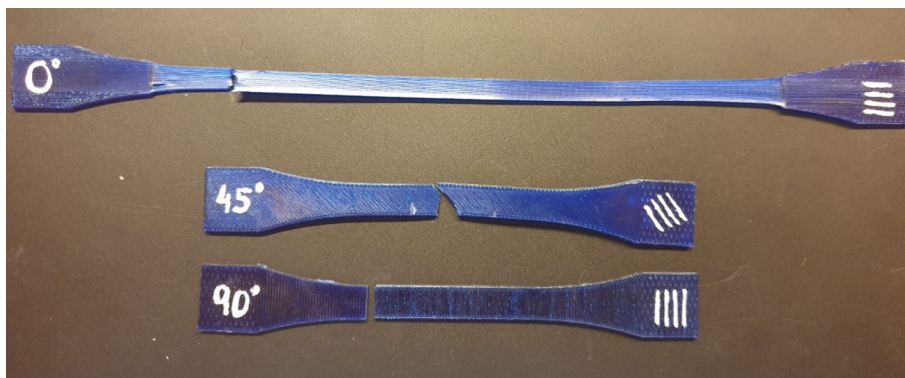
Figure 13: PETG tested specimens after failure.
