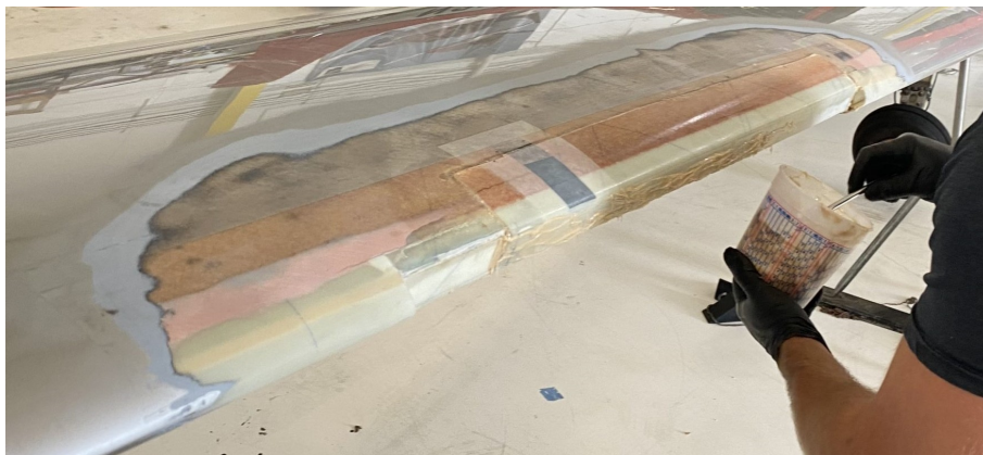
Figure 2.21: Adhesive application on a wing structure for a composite bonded repair (TCA, 2022).
