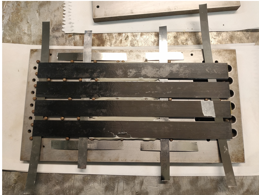
Figure 3.11: Specimens after joining substrates.
