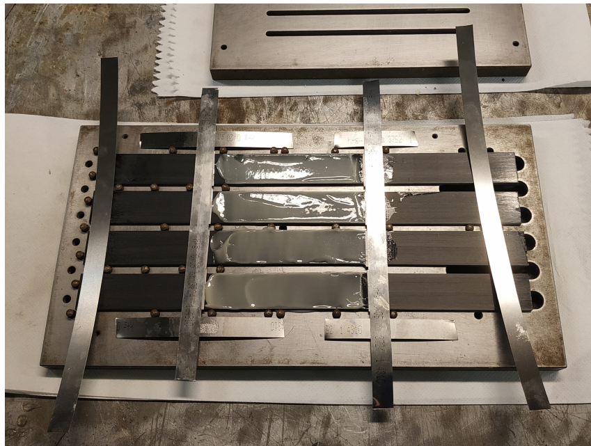
Figure 3.10: Substrates after adhesive application.
