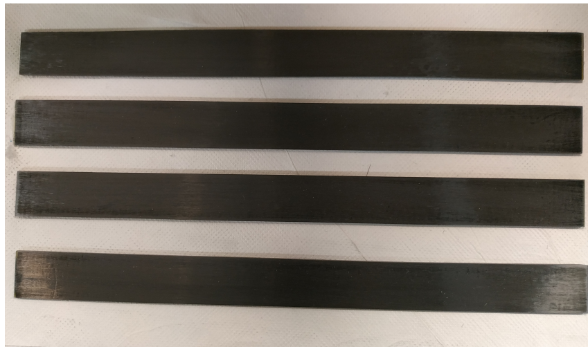
Figure 3.6: Substrates after surface preparation.
