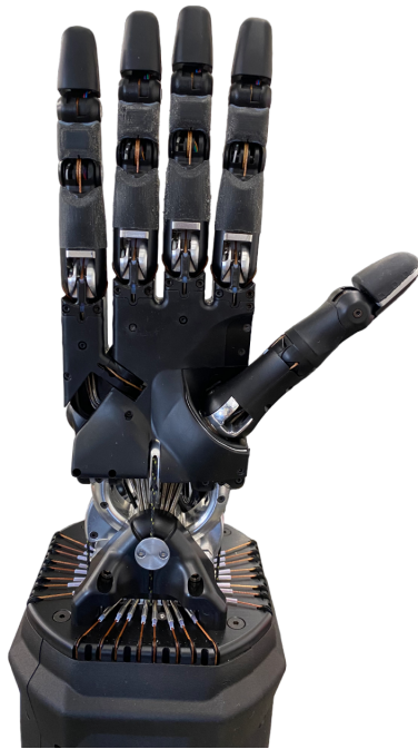
Figure 2.4: Real illustration of Shadow Dexterous Hand.
