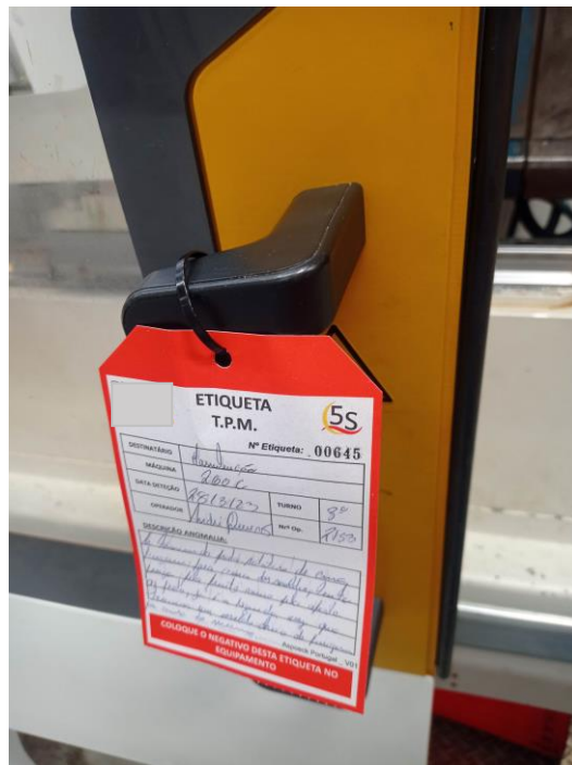
Figure C-2 - Example of a label assigned to maintenance.
