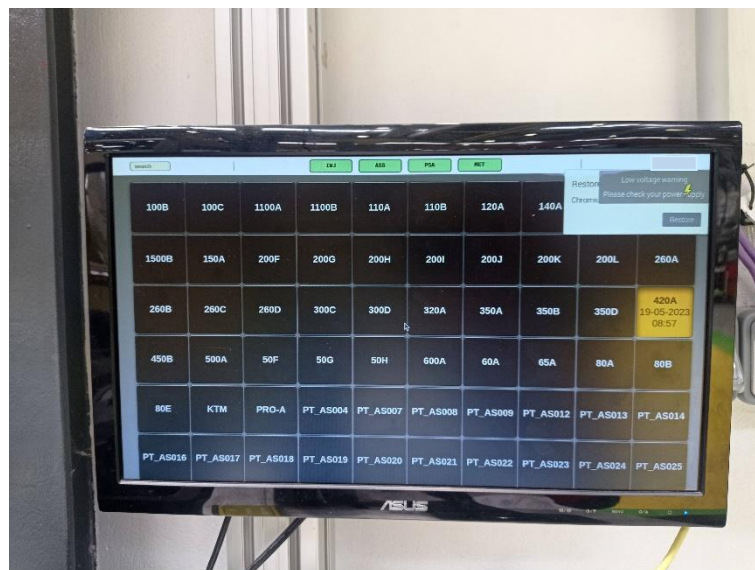
Figure 3.2 - TV that indicates the state of the equipment.
