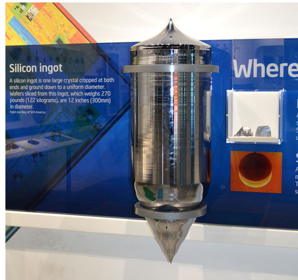
Figure 4.2: A silicon ingot at the Intel Museum ([3] under the Creative Commons Attribution-Share Alike 3.0 Unported license)
