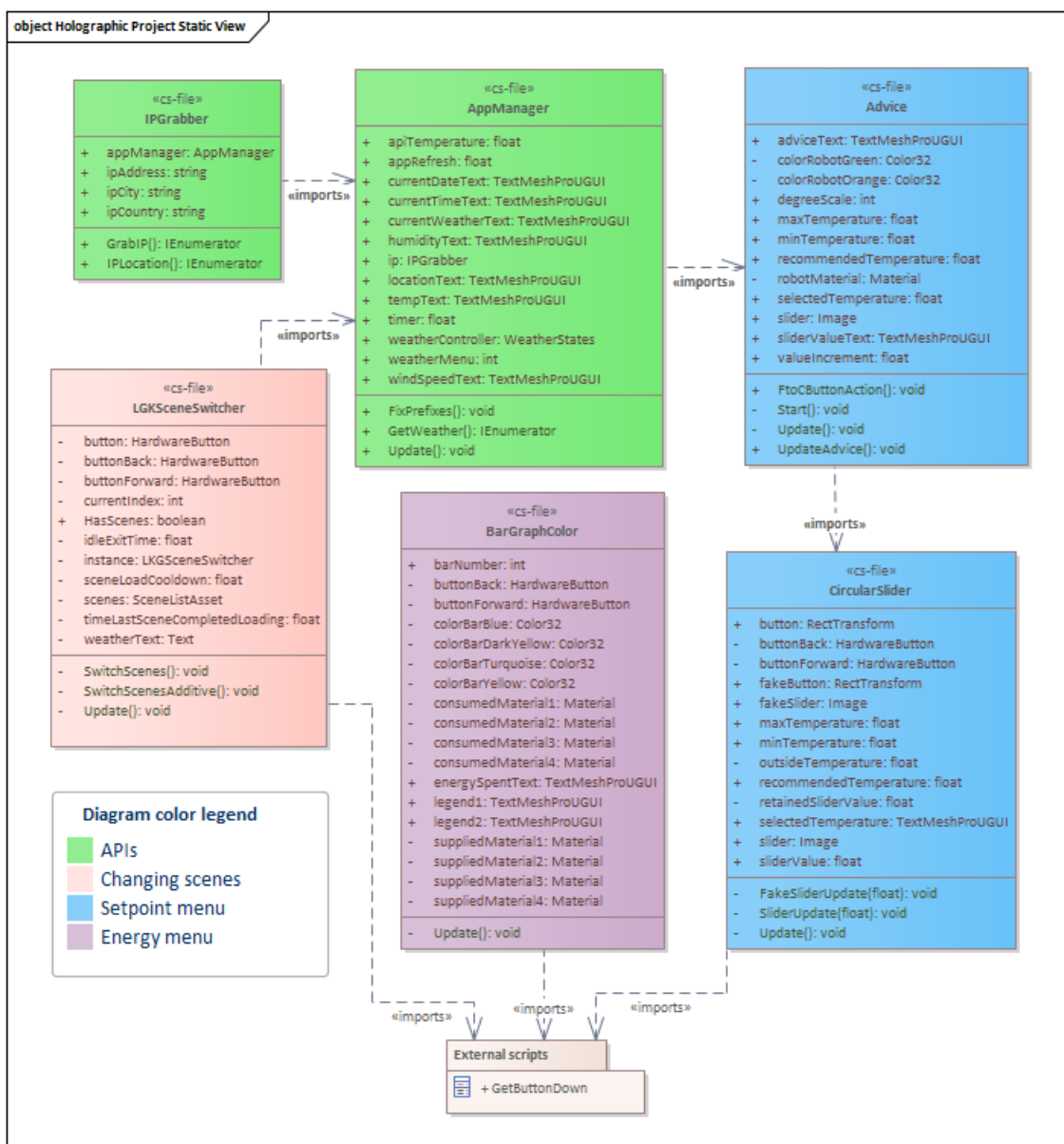
Figure 5.7: Holographic prototype architecture
