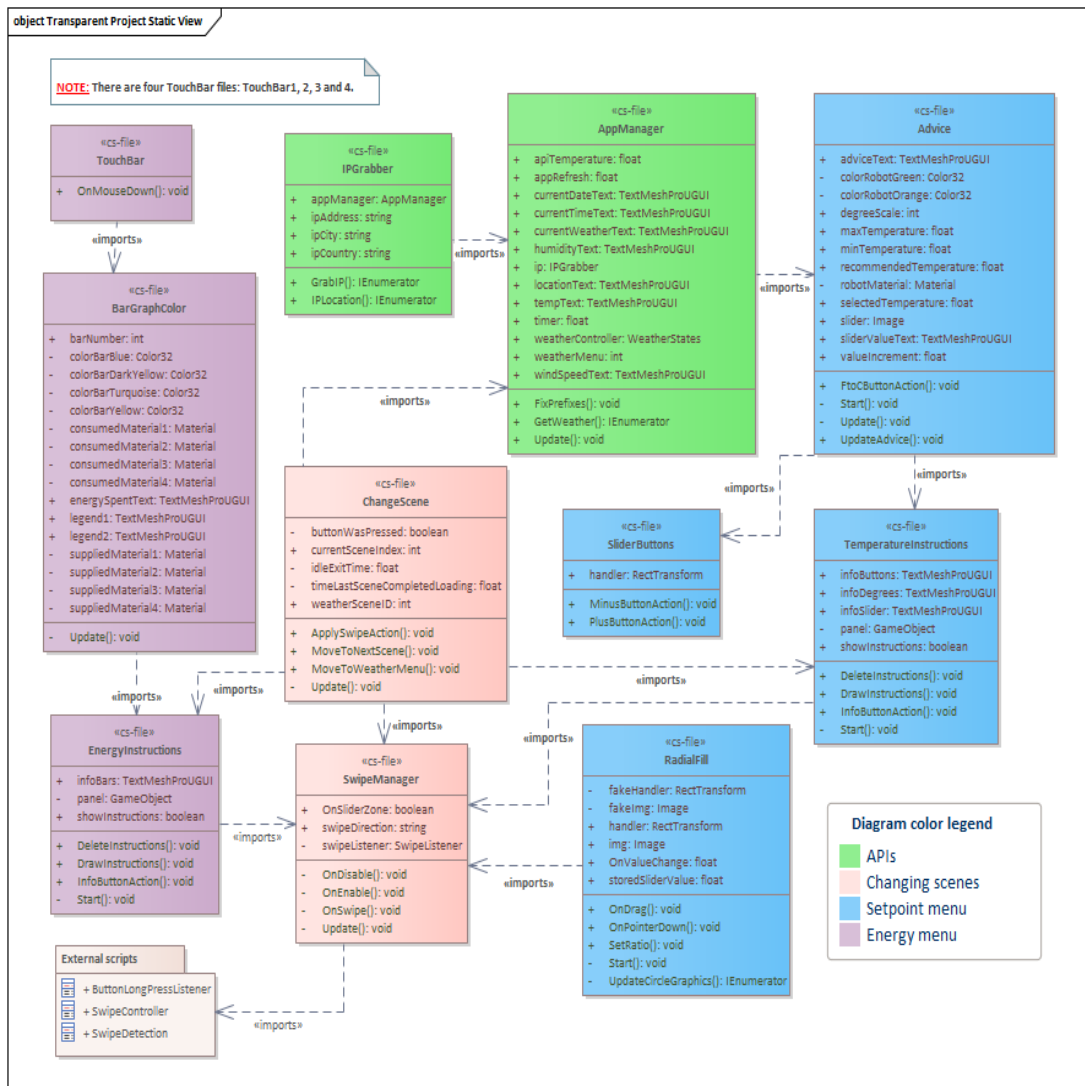
Figure 5.8: Transparent prototype architecture
