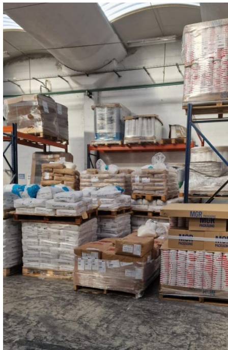
Figure 24 - Example of obstruction to rack access
