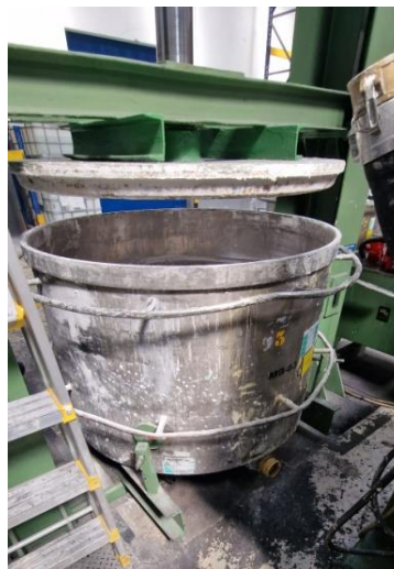
Figure 21 - Removal of the mobile tank during setup
