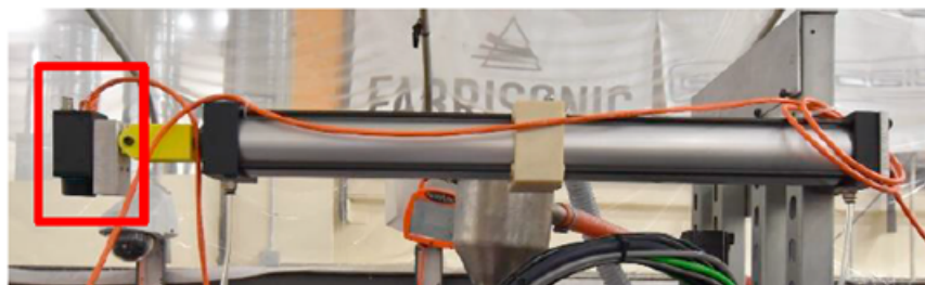
Figure 2.7: Camera setup on the pneumatic arm [19]
