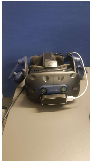
Figure 4.2: Headset used with LEAP Motion Device attached
