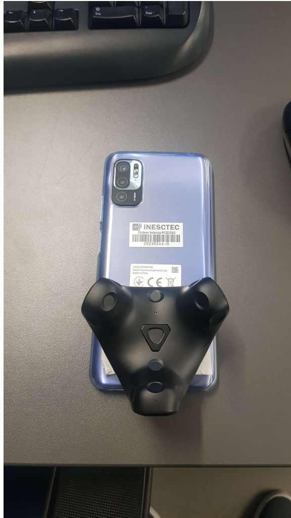
Figure 4.3: Positioning of the tracker attached to the smartphone
