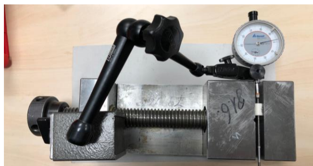
Figure 40 – LSN backlash characterization
