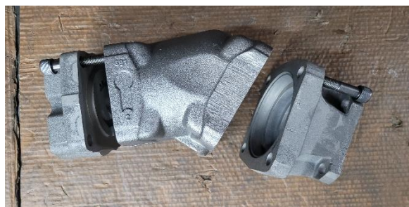
Figure 26 - Pump Housings for BIP (Rear Cover, Middle Housing, Fixation Housing)
