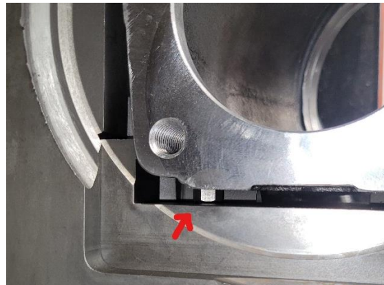
Figure 32 - Locator Pins for Supporting BIM Middle Housing
