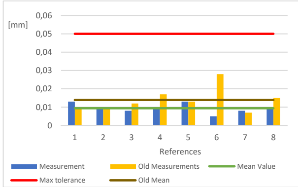
Figure 80 - Old vs New Flatness Tolerance Measurements Front Face
