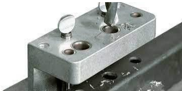
Figure 13 - Jig with bushings used in drilling operation [30].
