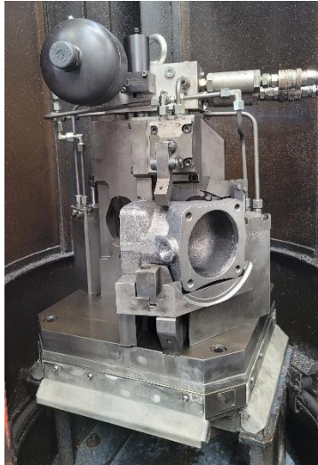
Figure 30 - P size middle housing old fixture
