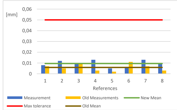
Figure 81 - Old vs New Flatness Tolerance Measurements Rear Face
