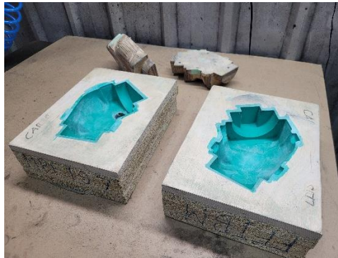
Figure 27 - Pattern and Mold of BIM Middle Housing
