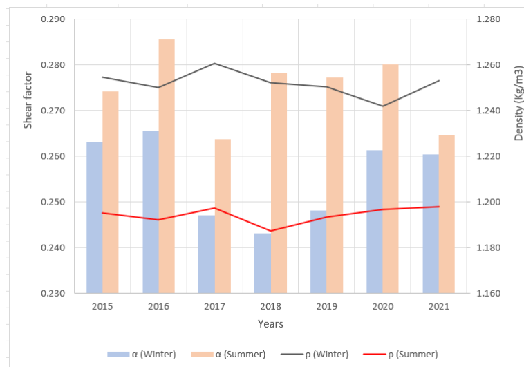
Figure 52: Shear factor and density values for Winter and Summer in each year
