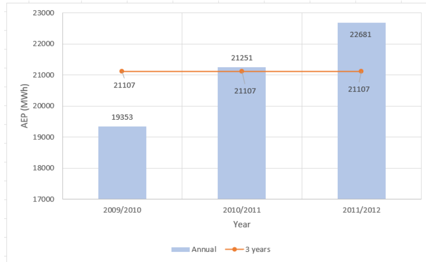
Figure 59: AEP values for each year versus AEP for 3 years calculation (Both from Time Series)
