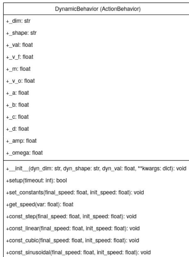
Figure 4.40: DynamicBehavior UML class diagram.
