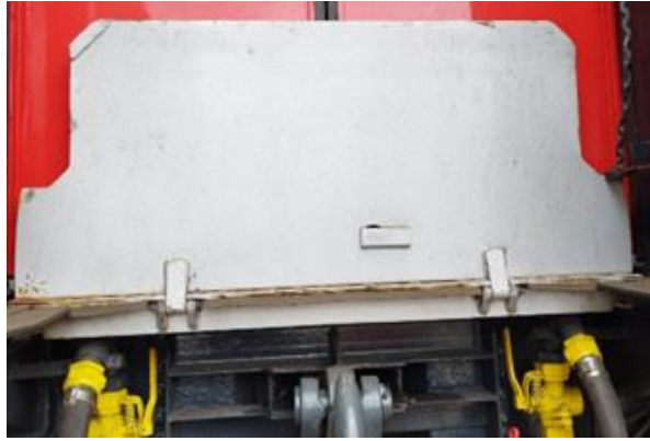
Figure 43 – Passage Flap (in raised position)
