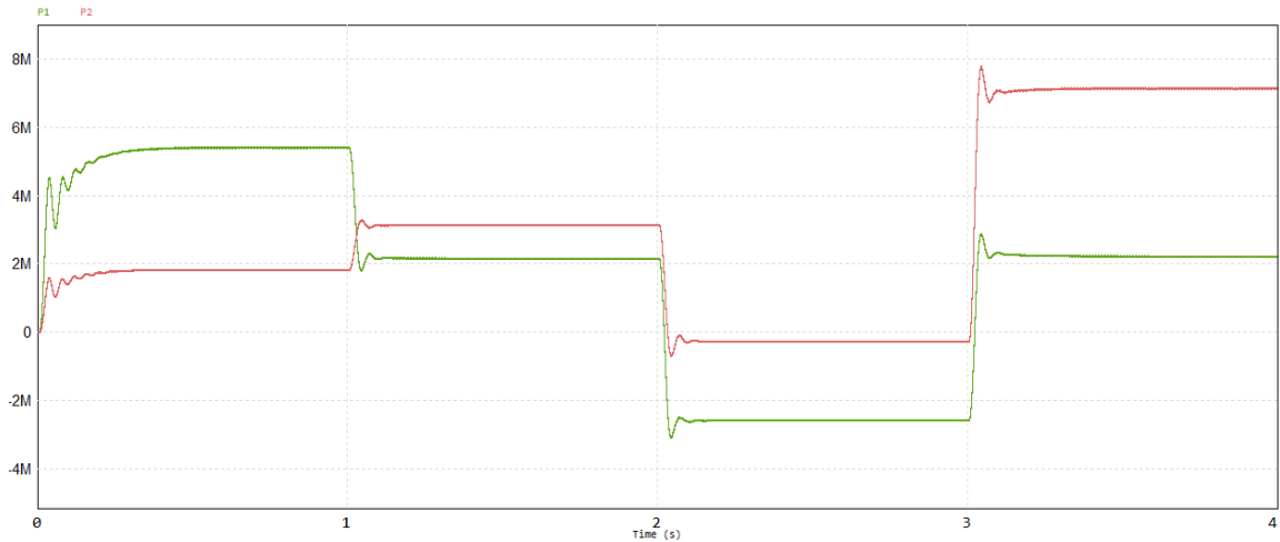
Figure 5.12 - Total power injected into the catenary by each substation in the first simulation of the first scenario.
