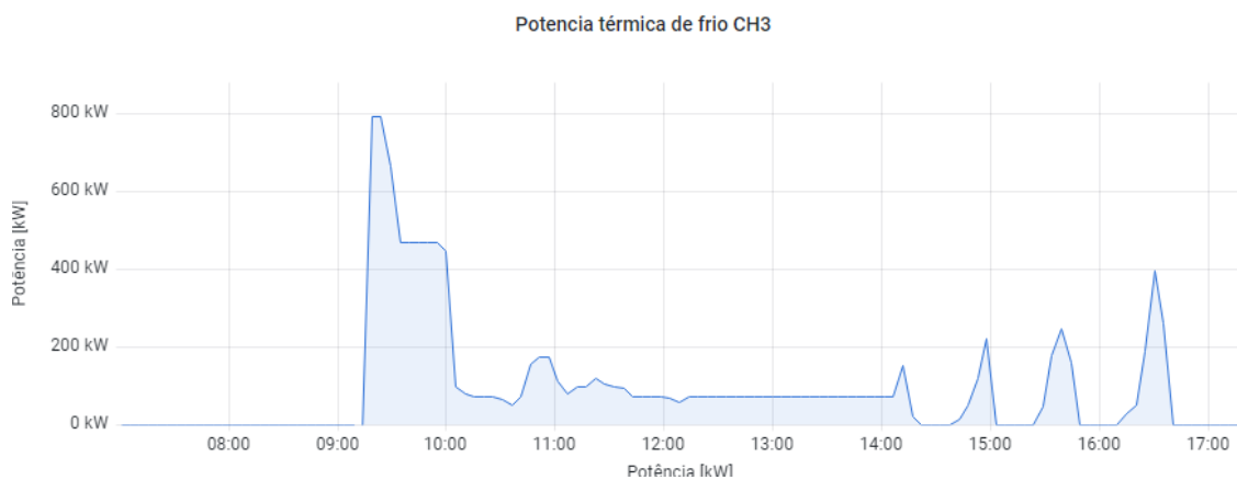
Figure 37- Chiller 3 Power output during Day 3.
