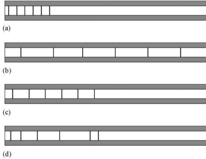
Figure 2.8: "Four cases of modelled crack spacings: minimum (a), maximum (b), mean (c), and random (d)." Figure and description from [41].
