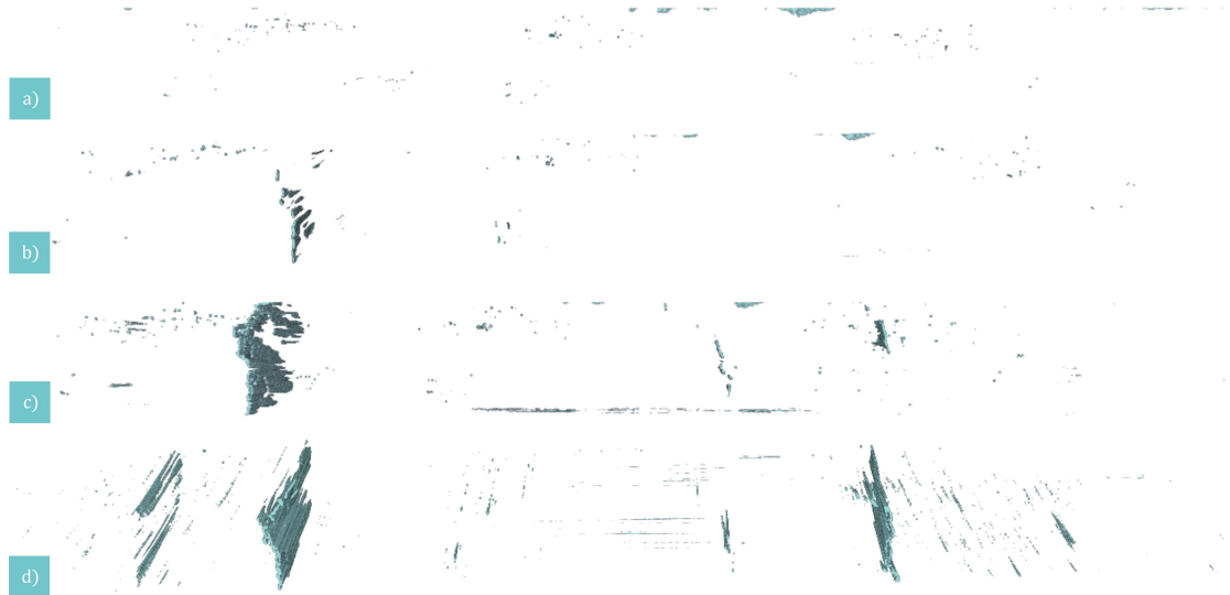
Figure 5.10: Representation of the damaged volume in the material Q4: a) 0% strain, b) 0.3% strain, c) 0.4% strain, and d) 0.5% for the view II.
