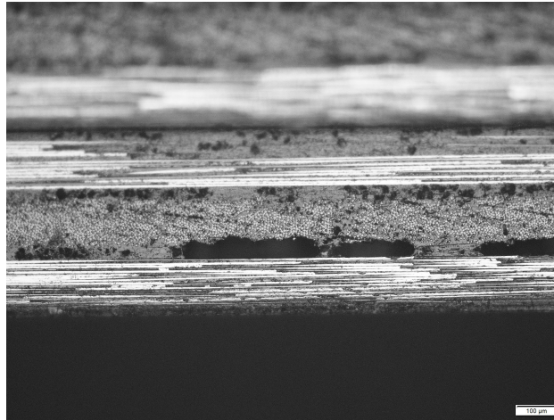
Figure 4.9: P1 laminate observed through optical microscopy.
