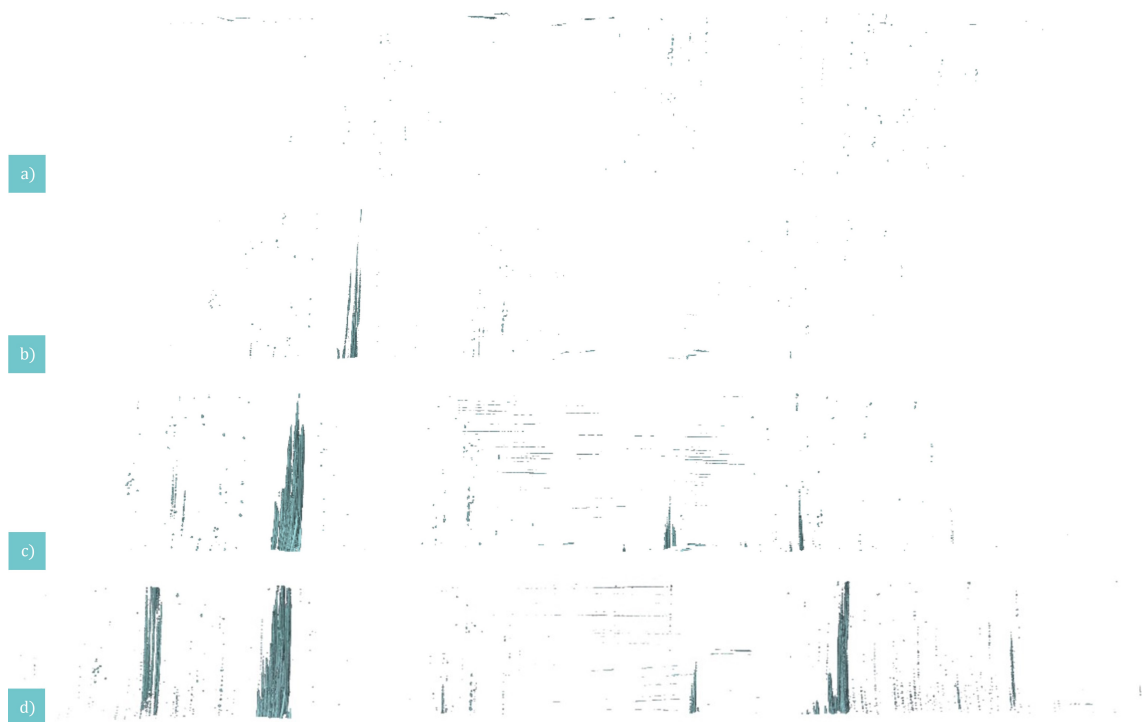
Figure 5.9: Representation of the damaged volume in the material Q4: a) 0% strain, b) 0.3% strain, c) 0.4% strain, and d) 0.5% for the view I.
