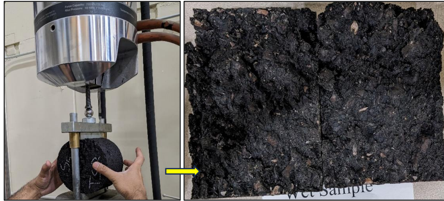
Figure 3.17 (a) TSR test setup; and (b) failure surface
