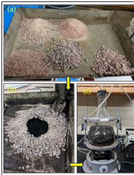
Figure 3.8 Determination of G_{mm} value (a) aggregates batching; (b) mixing aggregates and asphalt binder; and (c) de-airing of loose mix
