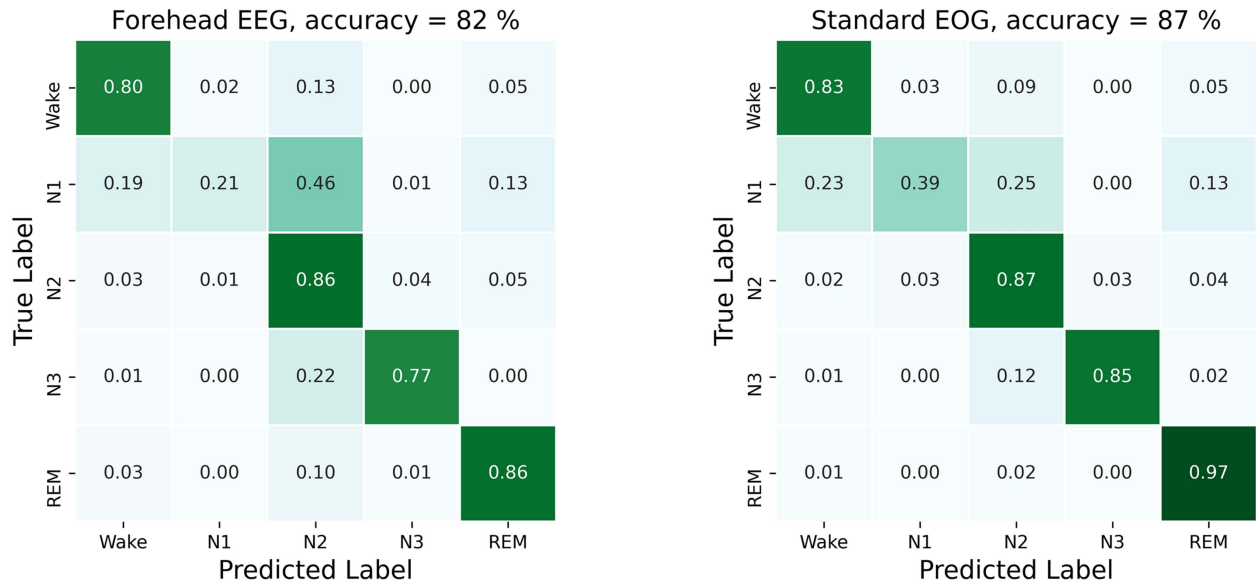
Fig. 5. Confusion matrices between the manual sleep staging (true label) and automatic sleep staging (predicted label) on home recordings. Forehead EEG (Fp1-Fp2) was recorded with the textile electrode headband and standard EOG (E1-M2) using medical-grade wet electrodes. Abbreviations: EEG = electroencephalography, EOG = electrooculography, Wake = wakefulness, N1 = Stage N1 sleep, N2 = Stage N2 sleep, N3 = Stage N3 sleep, REM = rapid eye movement sleep.
