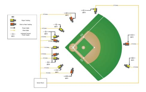
Figure 11: Typical Layout of Hawk-Eye Camera System (Jedlovec, 2020)
