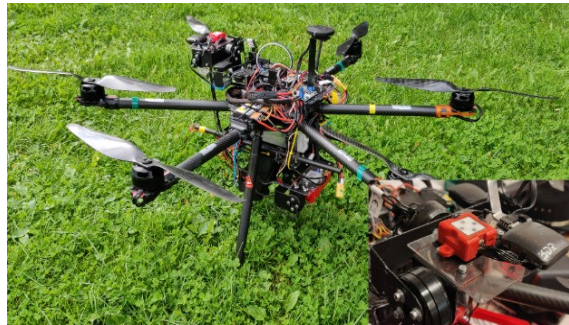
Figure 3. The UAV and the gimbal for the multispectral cameras light sensor (small figure). The gimbal helps the sensor to point nadir during the UAV flights.
