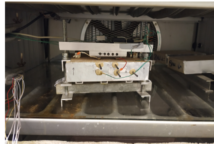
Figure 1. (b) Three specimens were used in the experiment being shown here. Sensors were attached to specimen a) to monitor the drying process; specimen b) was a reference specimen which was being used to determine the drying curve by means of weighing; and specimen c) was used to determine the moisture content of the wood at different depths by means of slicing.
