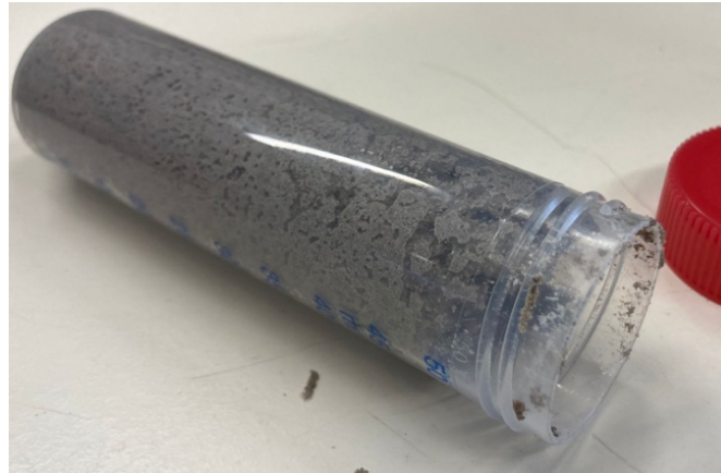
Figure 34. The hibernation test unit. A 50ml centrifuge tube filled with artificial soil.
