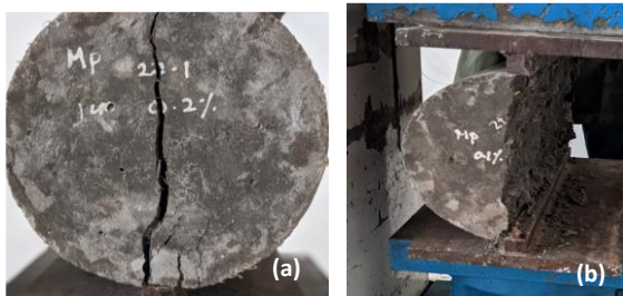
Fig.10 – Failure of cylinder specimen with and without fibers
