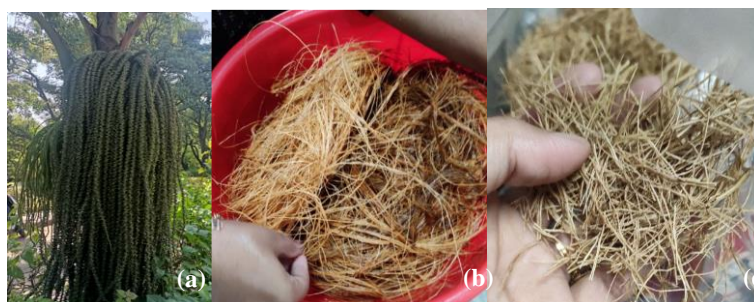
Fig. 1 – Caryota urens Fiber (a) Raw fiber (b) processed fiber (c) cut fiber
