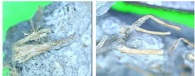
Fig. 11 – VMS images of fibers arresting the splitting cracks
