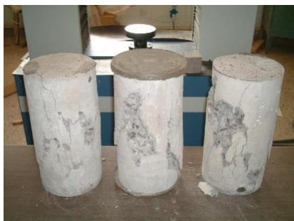
a- failure modes of concrete specimens (pozzolanic aggregate concrete).
