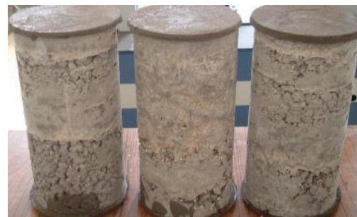
Fig. 14 – Case of segregation of concrete with pozzolanic aggregates.
