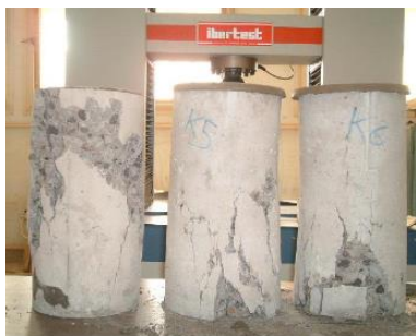
Fig. 13 – Mode of failure of concrete specimens (concrete with pozzolanic aggregates).
