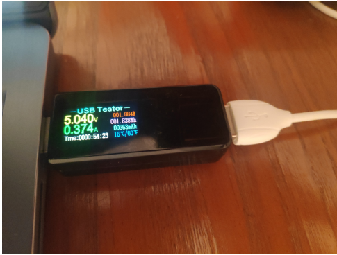
Fig. 6. An Atorch USB Tester was used to measure the energy consumption of running ML algorithms on the Raspberry Pi 4 Model B.
