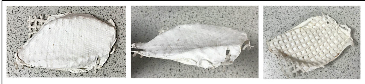
Figure 32 Composite 3D structure made from Varaform and electrospun PU fabric32
