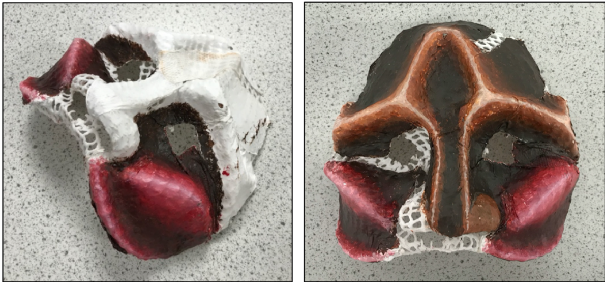
Figure 36. Testing the effectiveness of using watercolour paint on electrospun PU fabric
