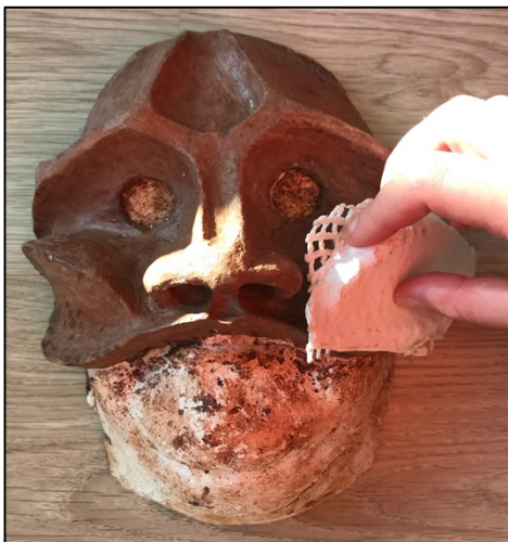
Figure 31 Activated Varaform is moulded over the clay mask mould, and electrospun PU fabric is stretched over, tensioned and bound to Varaform
