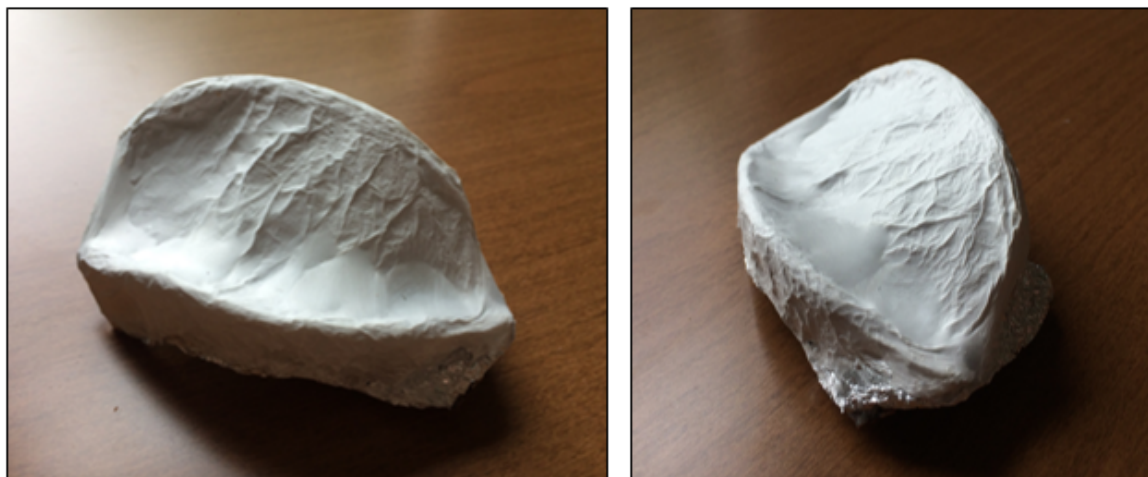
Figure 27 Electrospun PU fabric structure sample using 3D collector covered with aluminium foil (sample B)
