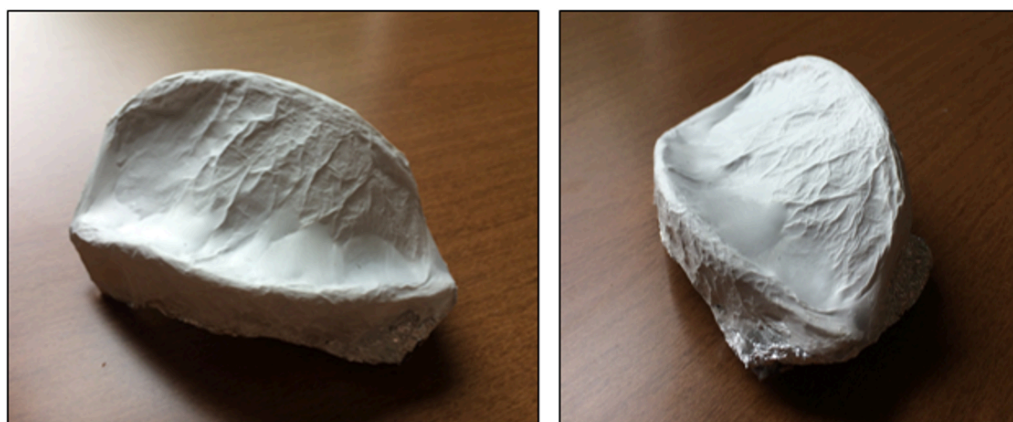
Figure 38 Electrospun PU fabric structure using 3D collector made out of wire mesh
