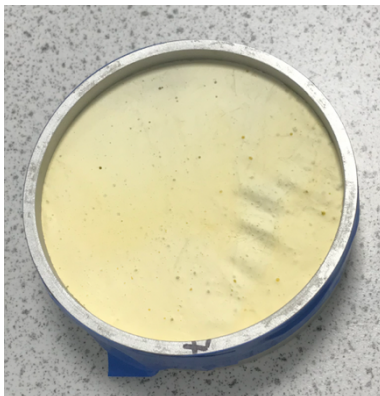
Figure 34 Electrospun PU fabric with added pigments before the electrospinning process
