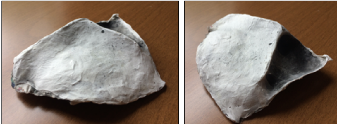
Figure 26 Electrospun PU fabric structure using 3D collector painted with electroconductive paint (sample A)
