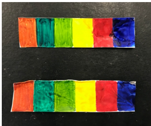
Figure 35. Testing the effectiveness of using watercolour paint on electrospun PU fabric
