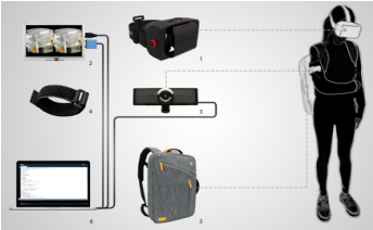
Fig. 1: The setup - 1. VR headset; 2. Touch Screen; 3. Wide-cam; 4. Fix band; 5. Backpack; 6. MacBook
