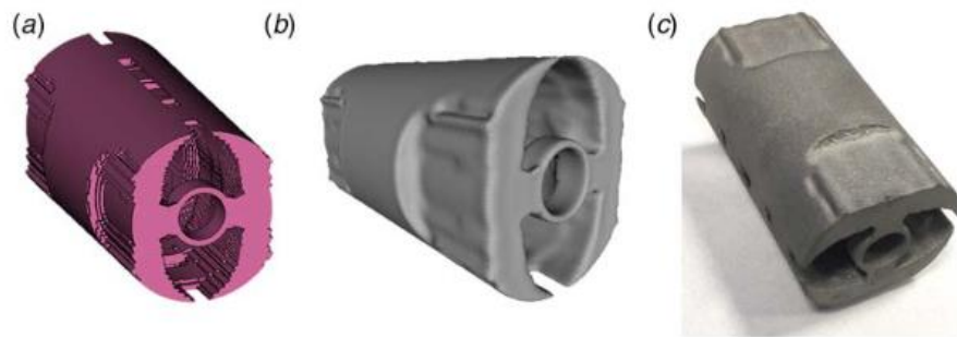
Figure 2-13 - Topology optimised PMM rotor showing optimisation results (a), post smoothing (b) and manufactured component (c). Reproduced from (39).
