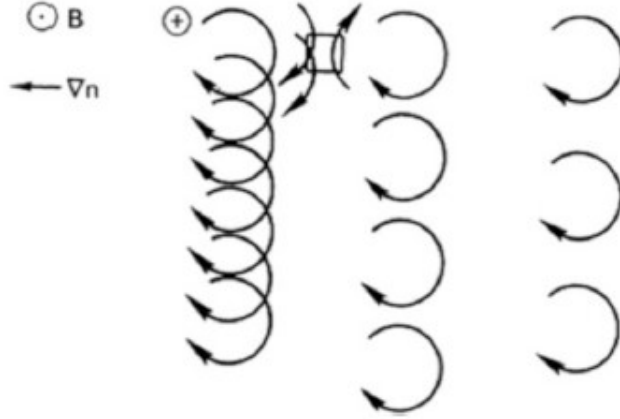
Figure 1.8: Schematics of the diamagnetic drift pointing downwards [15]
