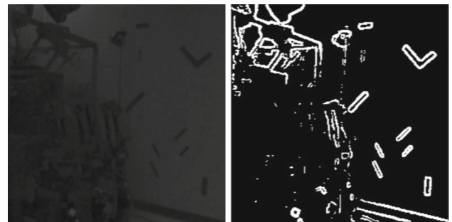
Fig. 12 An intensity image (Left) and its edges (Right) captured via D445 at 4ms exposure (Color figure online)
