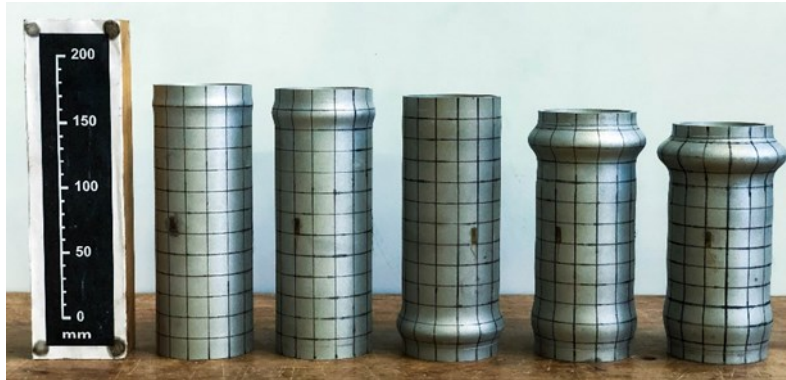
Figure 4.8: Deformed CHS stub column test specimens, with increasing wall thickness from left to right
