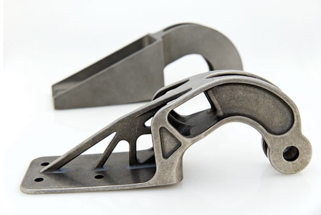
Figure 2.3: Original HC101 steel (top) and topologically optimised Ti-6Al-4V (bottom) nacelle hinge brackets produced by AM for Airbus A320 airliner (Tomlin & Meyer, 2011)
