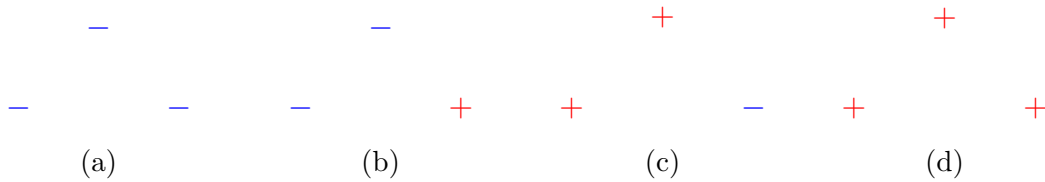
Figure 3.2: A set X of three points in \mathbb{R}^2 that is shattered by linear classifiers. Subfigures (a)-(d) represent different dichotomies on X ; note that (b) and (c) are not the only labellings with one and two positively labelled points, respectively, but the other cases are symmetric.
