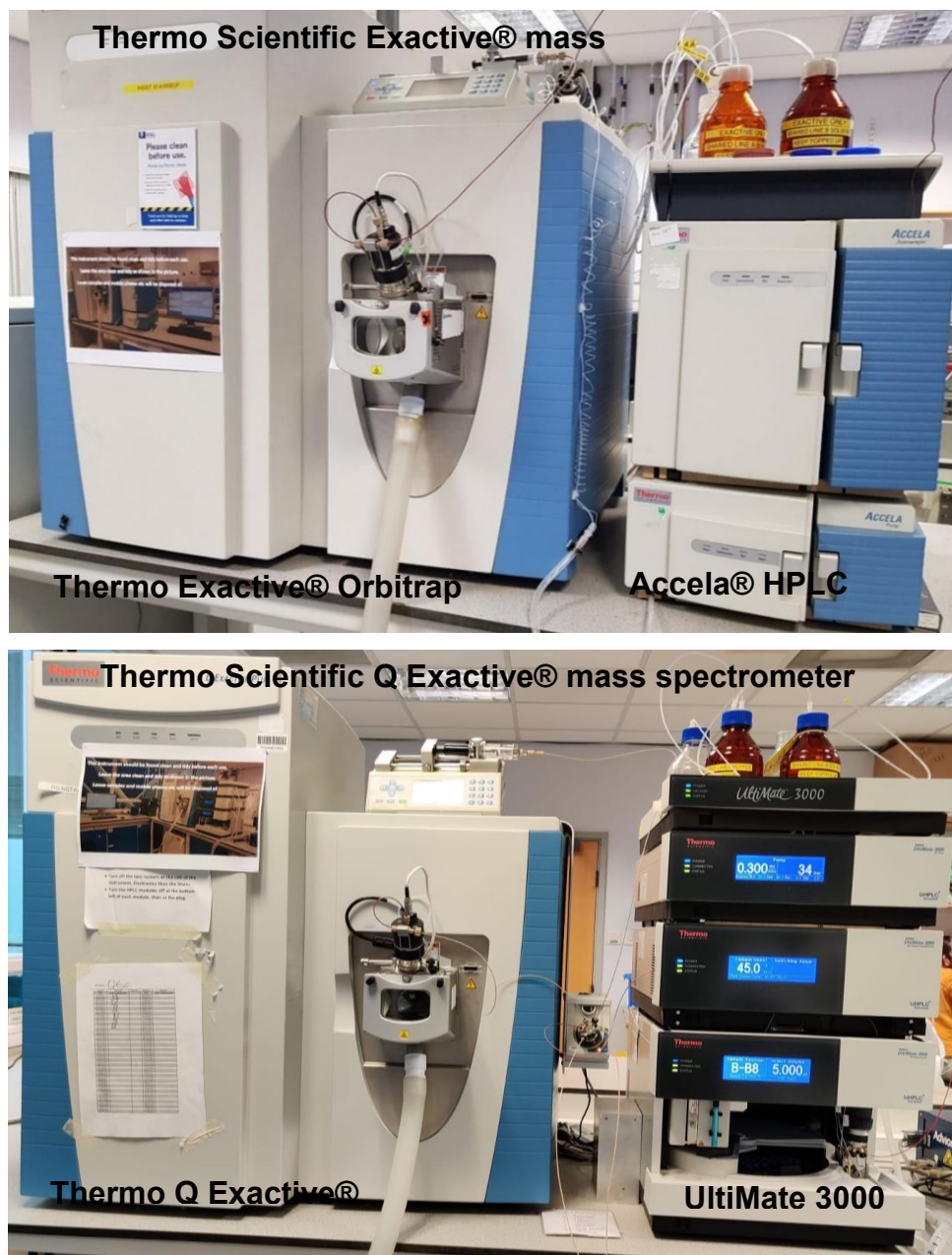
Figure 2.1: The Exactive Orbitrap Mass Spectrometer and Q Exactive Orbitrap Mass Spectrometer, setup used for LC-MS analysis.
