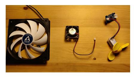
Figure 15: Left to Right: 120mm 12V Fan, 40mm 5V fan, GROVE 5V Mini fan.
