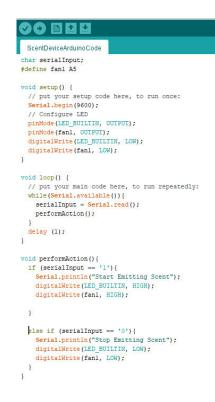
Figure 24: The code in Arduino can be seen here which tells the fan to spin if it receives a value of 1 from Unreal Engine 4, or stop spinning if it receives a value of 0.
