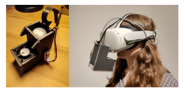
Figure 21: Left: The physical prototype device demonstrating how the Seeeduino nano is attached. Right: The prorotpye attached to an Oculus Quest 2
