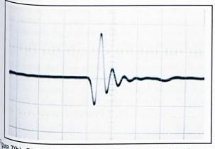
$\frac{Q_{He}}{M_{He}}$  7(b): Observed pulse waveform Vertical axis = 0.1v/div vizontal axis = 0.5µs/div
