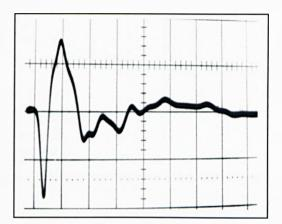
Figure 2.10(b): Measured pulse by practical measurement system. Vert. axis =10mV/div Horiz. axis = 0.5 µs/div
