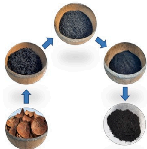
Fig. 2. Formation of coconut shell ash from the coconut shells.
